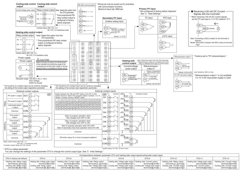
The types of control output, "relay output" and "voltage pulse output" shown in the table above refer to those of time proportional control.
