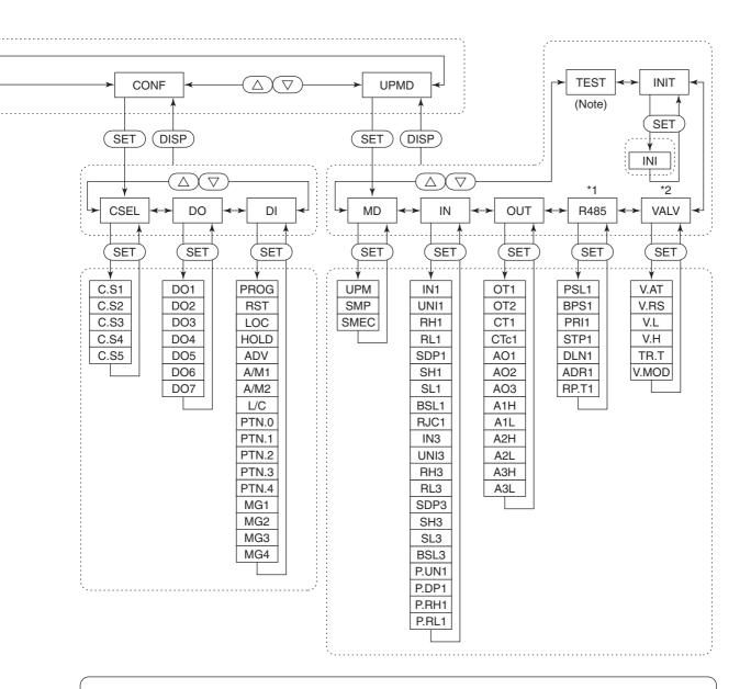
Note: The parameter items shown on the [TEST] submenu of the setup parameter setting display are to be used by Yokogawa service personnel to check the controller functions. User cannot set or change these parameters.
