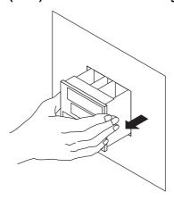
5. The location and number of the relays differ depending on the model code of the UP550. Confirm the location of the control output relay to be replaced before pulling out the relay.
