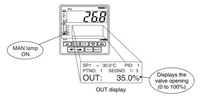
Note: The output high limit (OH) and output low limit (OL) do not restrict the manual output of position proportional control.
