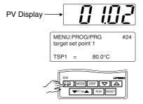
**12.** Press the △ or ▽ key to display the required setpoint.
