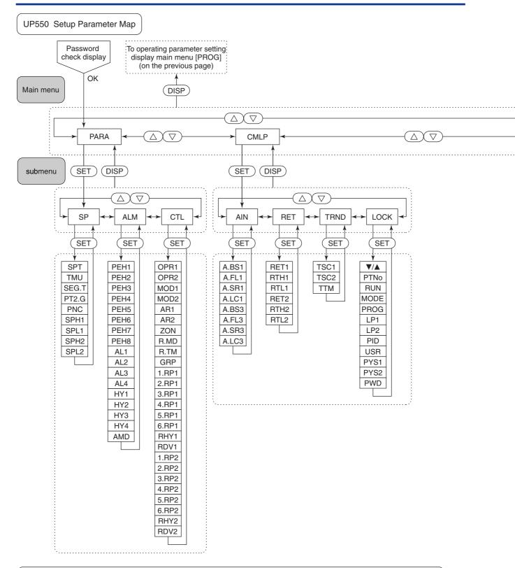
Pressing the DISP key once when a parameter setting display is shown retrieves the submenu of that parameter setting display.
