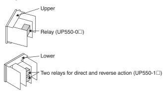
6. Pull out the relay to be replaced.
