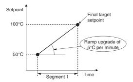
To change the temperature linearly over a minute, set the TMU parameter to "mm:ss" (minute and second) before you begin programming.
