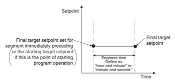
For example, configure segment 1 so the temperature rises in increments of  $5^{\circ}$ C per minute from  $50^{\circ}$ C to  $100^{\circ}$ C, as shown in the figure below.
