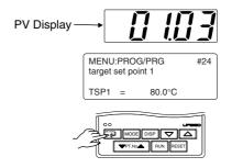
44. Press the △ or ▽ key to display the required setpoint.
